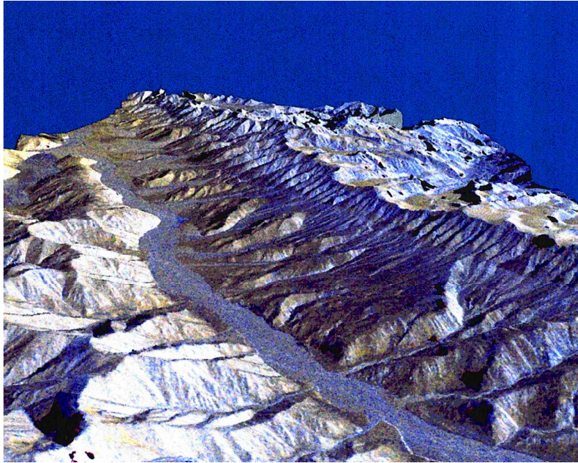
Fig. 3 Perspective view of the Karakax valley in Tibet created by combining two radar images using interferometry.
